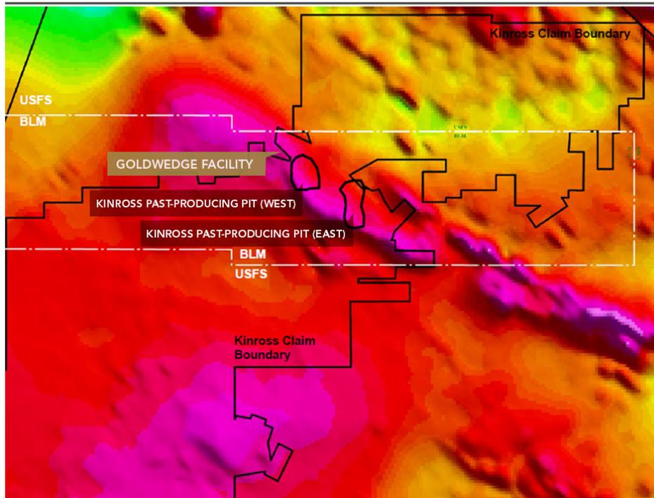
**Figure 4:** Airborne magnetic survey data (Re: Manhattan Divestment Proposal document – Kinross Gold Corp. October 21, 2016). The magnetic anomalies display the probable structural trends of the mineralized sheared metamorphosed interbedded limestones, argillites and phyllites of late Cambrian age.
