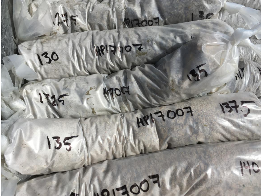
Figure 3 – Sample bags representing 2.5 core intervals from drill hole HP17007
