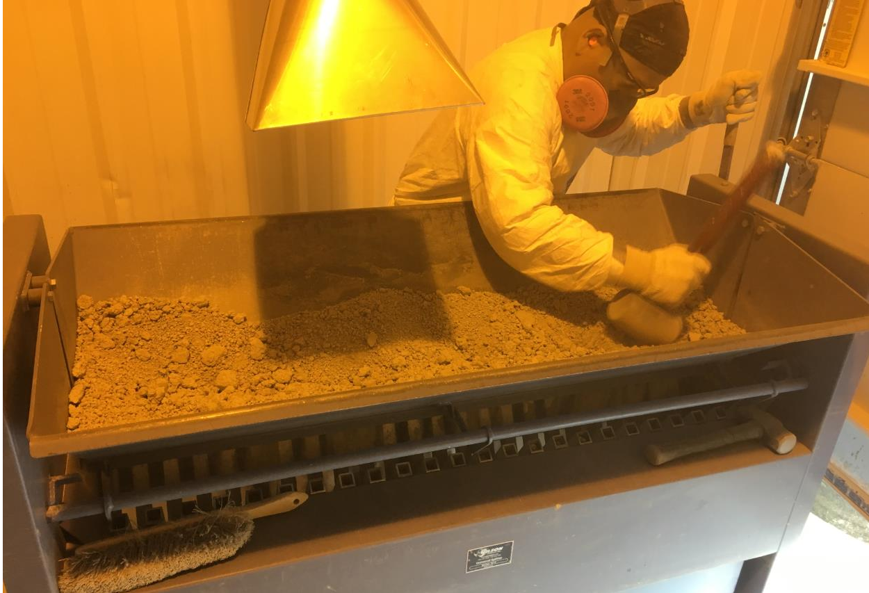
Figure 4 – Disaggregating sonic drill samples in the large-capacity Gilson splitter
